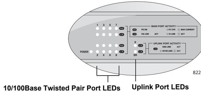
Figure 3. Port LEDs
