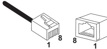
Figure 21. RJ-45 Connector and Port Pin Layout
